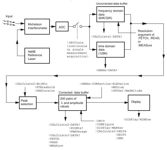
After collecting the uncorrected data, the Agilent 86122A searches the data for the first 1000 peak responses.
