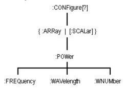
The CONFigure query returns the last configuration setup by CONFigure. The instrument returns a string that represents the current configuration of the instrument. The returned string is in the short command form, and returned values are in base units as in the following examples.
