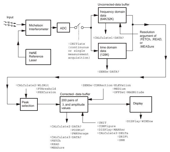
After collecting the uncorrected data, the Agilent 86122A searches the data for the first 1000
